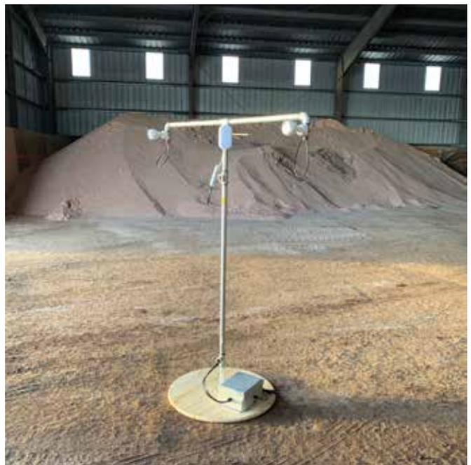
Fixed-camera poles enable bulk solids inventory monitoring in structures.
