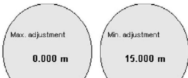
To perform the adjustment, enter the distance with full and empty vessel, see the following example:
