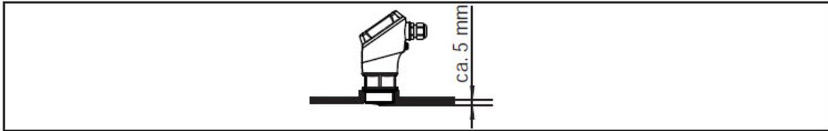
*Fig. 9: Thread mounting*
