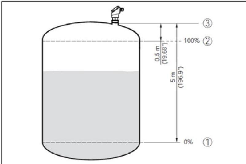
Fig. 16: Parameter example, Min./max. adjustment
