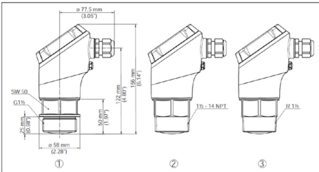
Fig. 20: Dimensions CNCR-230
