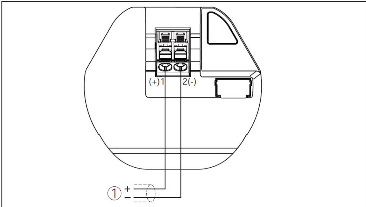
Fig. 12: Connection compartment CNCR-230
