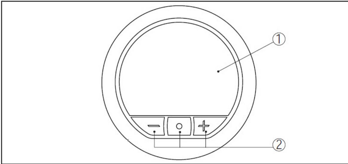
Fig. 13: Integrated display and adjustment unit
