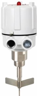
Rotaries are a familiar and common device used for high or low-level point level indication in bins, tanks, and silos. Rotaries are versatile enough to use in nearly any material from powders and granules with a minimum bulk density of 2 lb/cu ft<sup>3</sup> to coarse, lump materials with bulk densities up to 150 lb/cu ft<sup>3</sup>.
