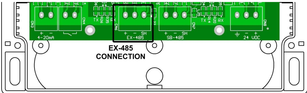
The EX-485 connection (CN6) is a three wire terminal block located near the center of the printed circuit board and is for connection to the Expansion RS-485 network. Two terminal screws marked + and – should be connected to the positive and negative wires of the RS-485 network cable. The third terminal
