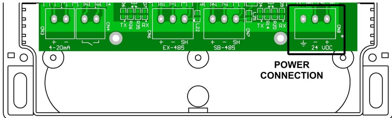
The power connection (CN8) is a three wire terminal block located on the far right. Two terminal screws marked + and – are for connecting to a 24VDC source, isolated from earth ground. See section 2.0 Specifications for power source requirements. Due to the low power requirements of this console, a 16 or 18 AWG wire would be sufficient for these two power connections.
