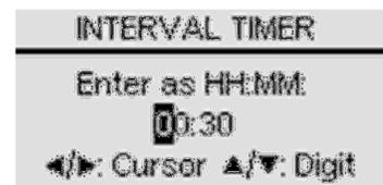
keys to select a digit by repositioning the cursor and the ▲/▼ keys to adjust the selected digit. Once all four digits have been entered, press the ✓ key.
