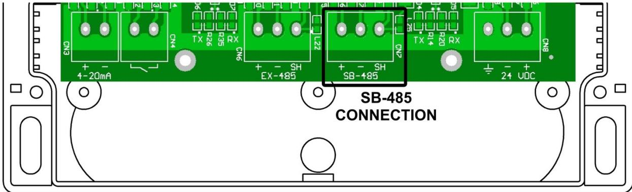
The SB-485 connection (CN7) is a three wire terminal block located near the center of the printed circuit board and is for connection to the SmartBob RS-485 network. Two terminal screws marked + and – should be connected to the positive and negative wires of the SmartBob network cable. The third terminal screw marked SH should be connected to the shield of the SmartBob network cable. Do NOT connect the shield to earth.
