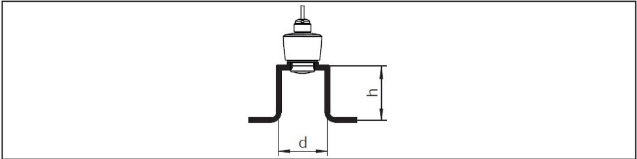
Fig. 8: Mounting the radar sensor with stand pipes
