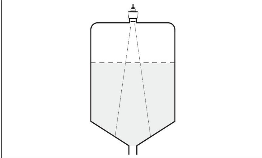
*Fig. 6: Mounting the radar sensor with conical bottoms*
