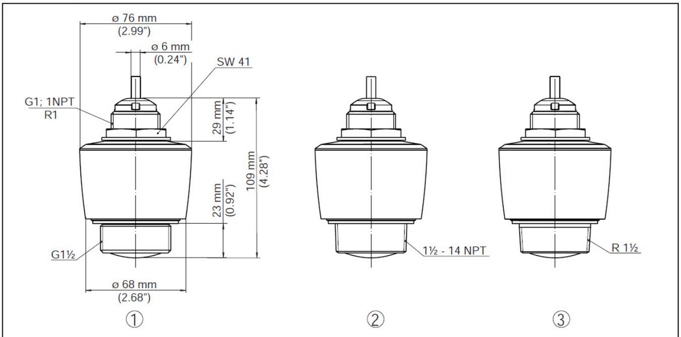
Fig. 13: Dimensions CNCR-110
