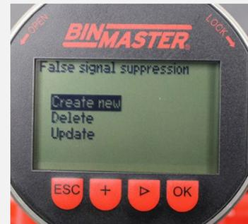
6. False signal suppression, use [▶] and [+] keys to set the actual distance from the sensor to the product surface
