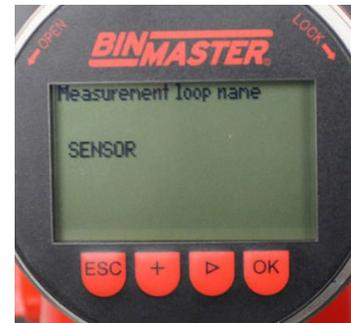
3. Medium, press [OK], scroll to Ballast/Pebbles Using [>] key (**do not change to any other medium**)
