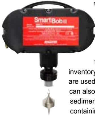
retracts while counting pulses that are converted to a level measurement. Measurements are programmed at predetermined time intervals to monitor changes in inventory over time. These sensors are used in solids or liquids and can also measure the level of sediment settled in a tank containing liquids.
