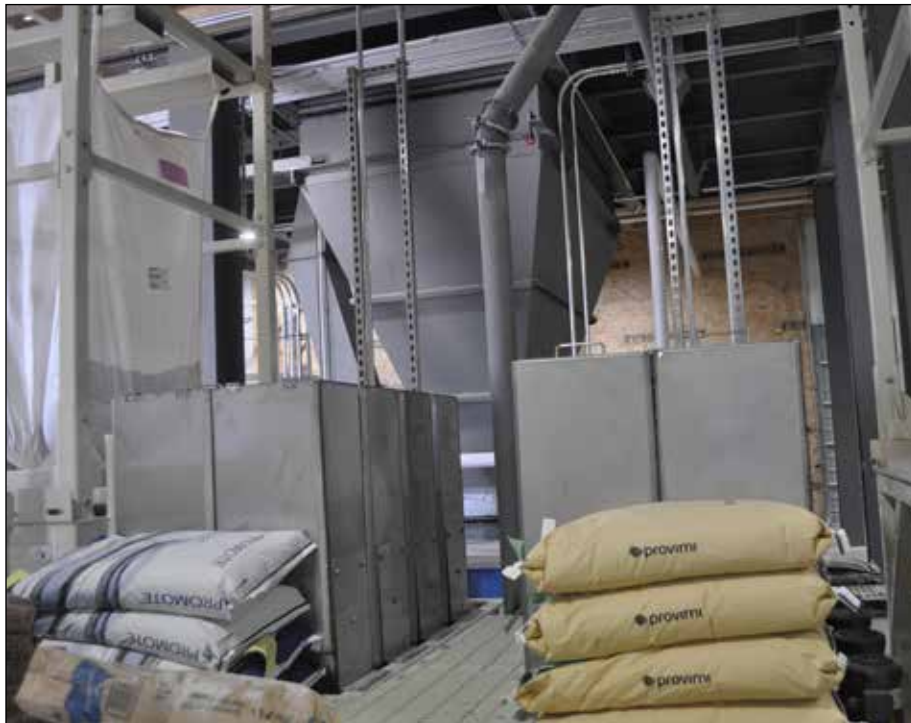
New Easy Automation 16-bin microingredient system supplies smaller ingredient amounts to the mixer.
