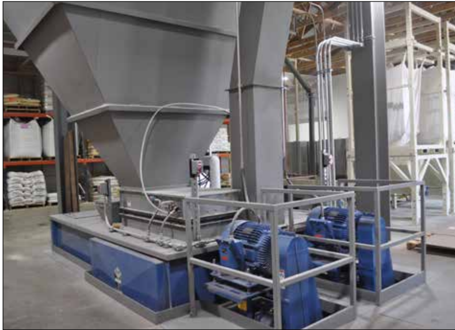
Ingredients are deposited into a batching scale, then to a 4-ton Scott double-ribbon mixer.
