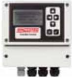
This compact, manually operated console can control up to 128 SmartBob-TS1 sensors with the push of a button. Individual bin heights are programmed to the console and measurements are displayed as distance to product, height of product, and percent full.
