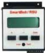
The RSU provides an external start input, a 4-20 mA current loop output, and a remote read-out of the measurement. The RSU allows for a simple interface between the SmartBob-TS1 sensor and a PLC or DCS system. The PLC/DCS initiates the measurement by providing a dry contact closure and then can retrieve the measurement from a 4-20 mA output.
